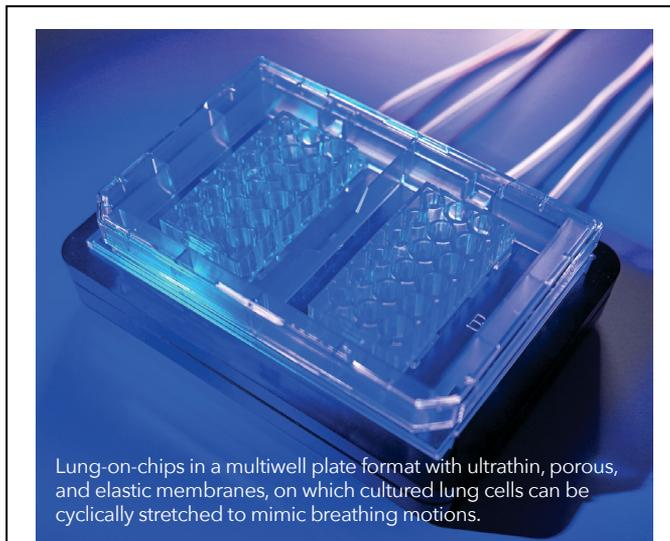
Lung-on-chips in a multiwell plate format with ultrathin, porous, and elastic membranes, on which cultured lung cells can be cyclically stretched to mimic breathing motions.
