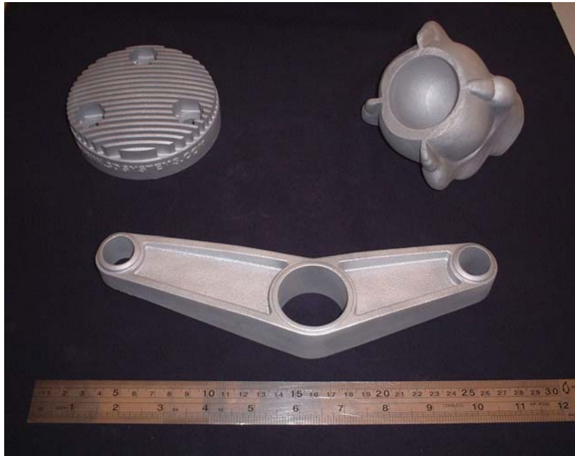
Fig S1. Aluminum parts made by laser sintering and infiltration. The ball and claw weighs approximately 950 g.
